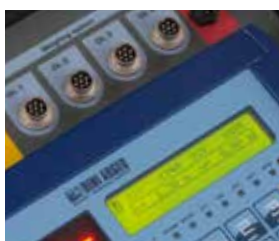
LCD BACKLIT DISPLAY able to show the weight of each platform and the centre of gravity.
